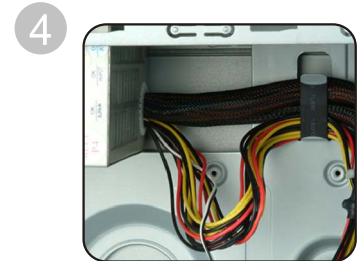
4 Unique PSU cable holder design
