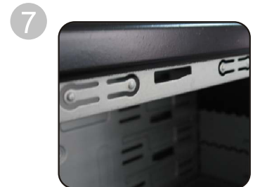
7 EMI springs to minimize EMI radiation
