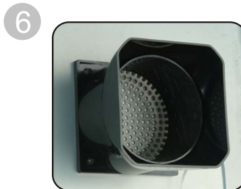
6 Intel CAG v1.1 Air Duct for extreme CPU cooling
