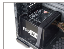
Velcro cable tie for PSU securing
