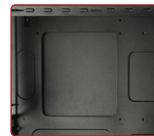
Cutout for CPU cooler maintenance
